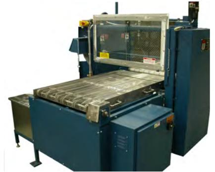
*Drawing compound coater specifically designed to fit between columns of a transfer press. It will accept various sizes of stock parts.*
