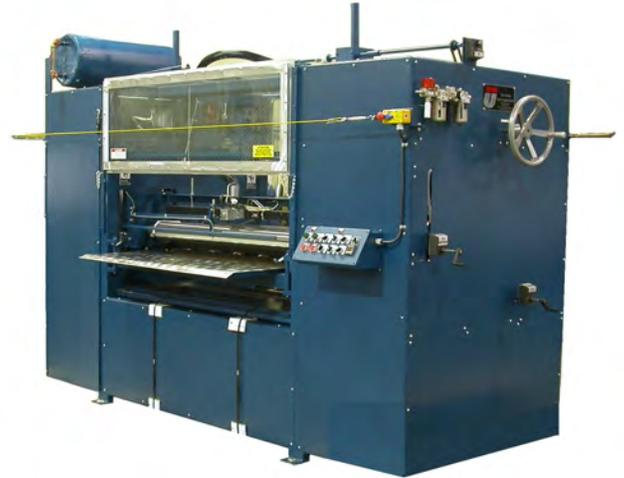
*Union Tool's Dual Head Series #15, Model A/D, 54" Hot Melt Roller Coater. A double-sided hot melt roller coater that, with a flip of a switch, can be used as a single side coater without any downtime. This is one of our most popular machines used in the RV Industry today.*
