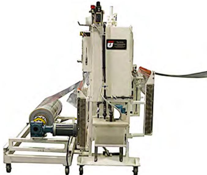
*Our plastic web roller coater draws web-feed (or roll -fed) plastic material from an integrated un-winder, coats it single or double sided with a silicone, anti-fog, or anti-static coating, then feeds it into a thermoforming press line.*
