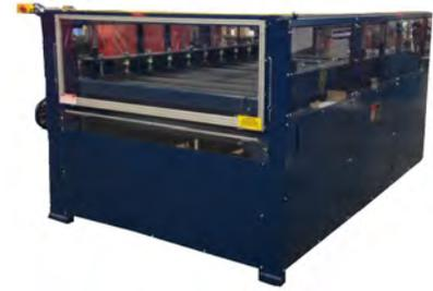
*Our Series 15, multi-nip rotary laminator is used to exert pressure to bond all constructed door panels together.*
