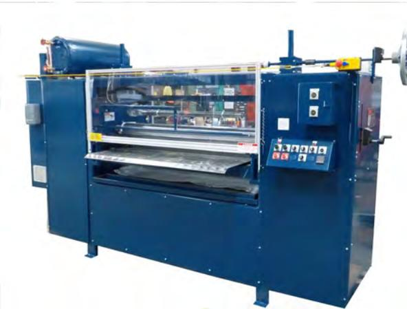
*Union Tool's Series #15, Model A, 54" Hot Melt Roller Coater. A double-sided hot melt roller coater that is designed to apply hot melt (PUR) adhesive to both the top side and bottom side of RV Materials.*
