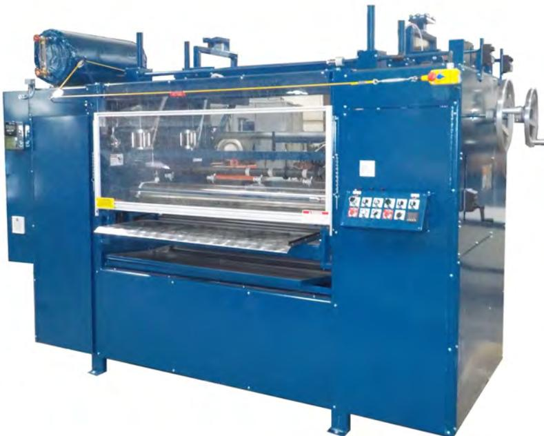
Union Tool's Hot Melt Roller Coater/ Hot Roll Laminator Combination Machine is an all-in-one type of machine. This machine combines the use of a hot melt roller coater, to apply hot melt adhesives, and a hot roll laminator, to laminate adhesive backed films, all under one framework machine.
