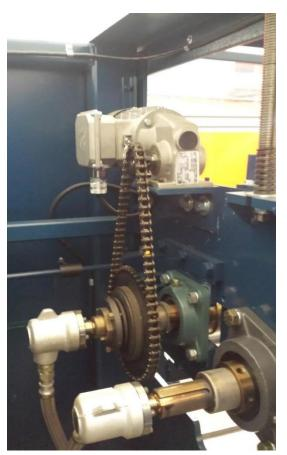
The clutch is adjusted by loosening the set screw that holds the outside tightening ring in place and then screwing the outside ring tighter.
