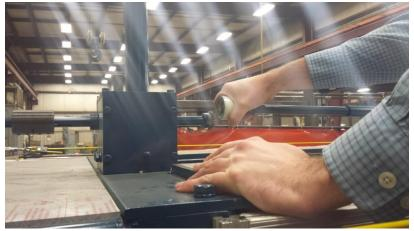
To parallel the rolls, the spring-loaded coupling that connects the shaft between the two vertical gear boxes must be pulled back. This will allow one side to be adjusted without moving the other side. It is often easier to adjust the hand wheel side so that you know how far you have opened or closed the gap to make the rolls parallel. To parallel the rolls we recommend using a .015 feeler gauge. When paralleling the rolls always make sure that the machine is turned off for safety purposes
