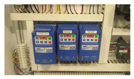
Union Tool coaters include AC variable speed drive controllers that control the speed of the rollers. The controllers are labeled to indicate the roll in which each controller is maneuvering. Variable speed ratios will depend on the specific series of roller coater.
