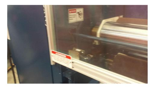
All Union Tool coaters incorporate sliding window guards. These window guards are located on the front and back side of the coater and are equipped with **magnetic sensors** so that the guards must be in place in order for the coater to operate. These guards are an important safety feature and provide the operators to run the machine in a safe manner.
