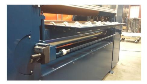
The doctor roll(s) is adjustable on a horizontal plane in relationship to the coating roll to control the amount of coating being applied. As the doctor roll is adjusted into the coating roll, less coating will be applied. As the doctor roll is moved away from the coating roll, more coating will be applied. The adjustment for the doctor roll is called a Unifeed. It is a single hand wheel that connects two (2) gear boxes that turn a screw moving the doctor roll on a horizontal plane.
